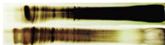
Figure 7: Top lane shows a gel over stained with FASTsilver™ and the bottom lane shows the same gel destained with Silver D-Stain™ and then restained with FASTsilver™, this allows more protein bands to be visualized.
