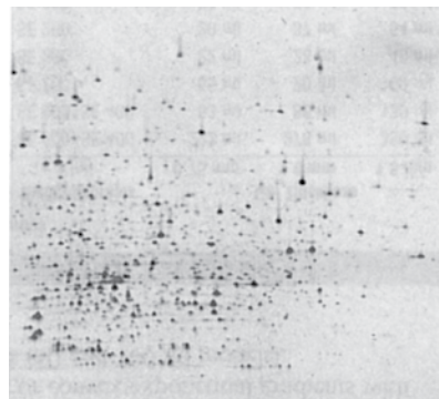
Figure 13: Treatment of protein samples with Perfect-FOCUS™ results in streak free, high spot resolution gels.
