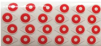
Sealing mats are available in 96-well round, 96-well square and 384-well square. The silicone patch is ideal for sealing individual wells or being attached to any surface to be used for withdrawal or injection of liquids.
