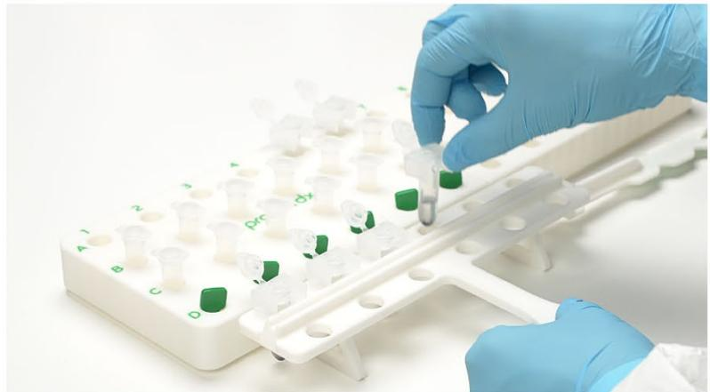
**Mixing:** The SmartLid Shaker provides a convenient solution for simultaneously mixing up to 12 samples at a time.
