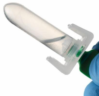
**2** Inverting the tube with the Magnetic Key inserted collects the Magnetic Beads onto SmartLid.
