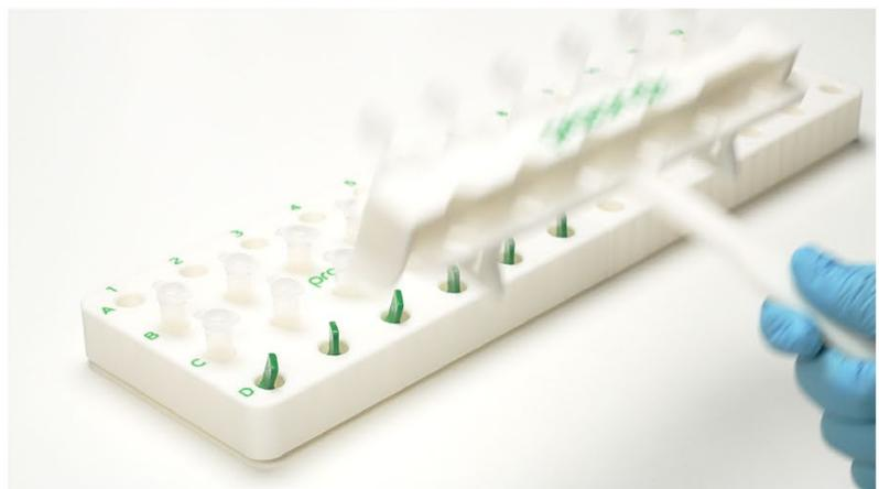
**Bead collection:** Inverting the SmartLid Shaker, with Magnetic Keys inserted, enables rapid and efficient Magnetic Bead collection.
