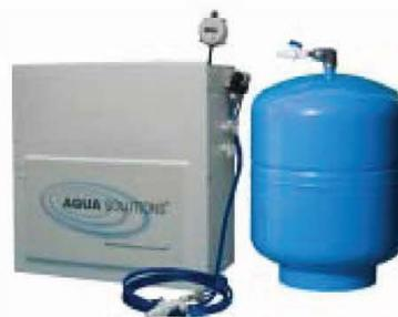
The systems include built-in 10 or 20 LPH reverse osmosis (RO) pretreatment to reduce operating costs by as much as 90%, while allowing the system to run on virtually any quality potable water. The RO purified water is stored in a 42-Liter pressurized storage tank.
