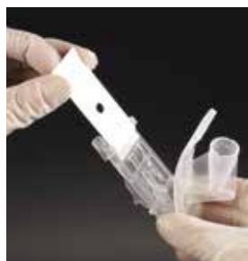
Place new filter onto microscope slide.
