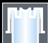
Sealed position for anaerobic cultures
