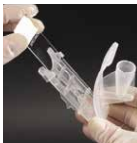
Insert microscope slide.
