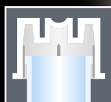
Loose position for aerobic work
