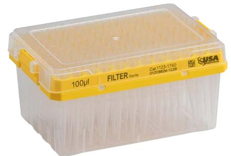
The transfer cover protects the filter tips while the unwrapped refill cassette is being placed into the rack.
