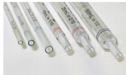
Serological pipets are color coded by volume for quick identification. Sterile, non-cytotoxic, and certified free of detectable RNase, DNase, and pyrogens.
