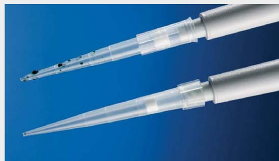
Comparison between pipetting viscous sample using standard tip (top) and TipOne RPT tips (bottom). Sample retention is dramatically reduced when using TipOne RPT tips.
