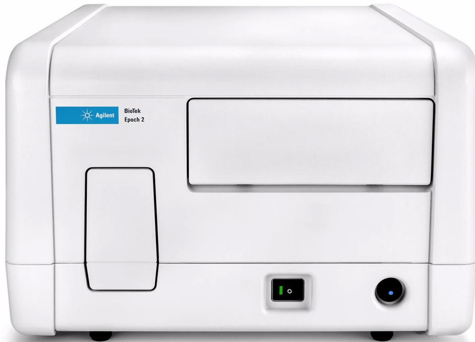
The BioTek Epoch 2 microplate spectrophotometer delivers excellent performance for UV-Vis absorbance measurements. Measurements can be performed in 6- to 384-well microplates, cuvettes, and in microvolume samples with the available Take3 microvolume plate. The broad wavelength range enables applications from nucleic acid and protein quantification in the low UV to microbial growth assays higher wavelengths.
