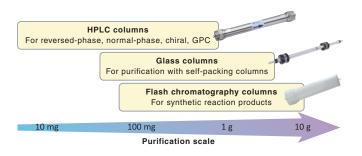
LC-Forte/R-II is useful for lab-scale preparative purification with HPLC columns, glass columns and flash chromatography columns. It is applicable for every modes such as reversed-phase, normal-phase, chiral and GPC.
