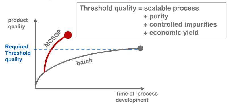
In order to achieve a required threshold quality with an optimized batch process, extensive process development has to be performed. Switching to MCSGP from a simple, nonoptimized batch process yields a superior product quality in a shorter time
