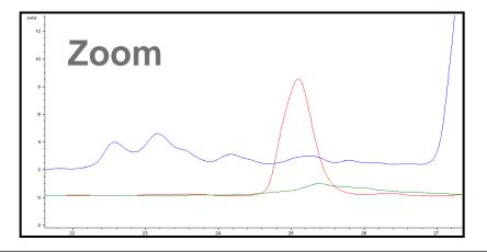
Blue: Feed Red: Side component by MCSGP Green: Side component by batch
