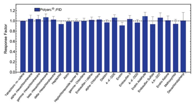
Response factors obtained for a 22-component organochlorine pesticide mixture using the Polyarc system.
