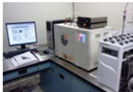
Multi column/multi detector GC for low level atmospheric gases
