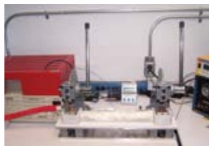
Custom sampling device for sealed container
