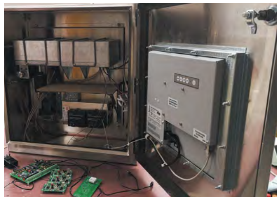
Custom Process Analyzer with NEMA Enclosure and Integrated Touch Screen PC
