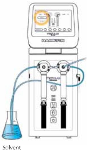
**Step 2.** Trigger the hand probe to fill a syringe with Solvent.
