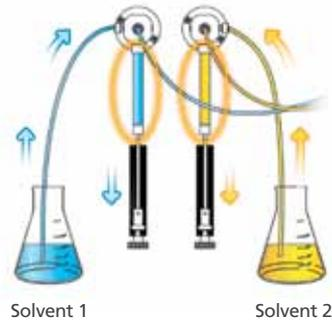
**Step 3.** Trigger the hand probe to dispense the left and right syringe into the same or separate vials.
