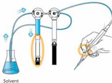
**Step 3.** Trigger the hand probe to dispense Solvent from the full syringe and fill Solvent into the empty syringe. One syringe is always filling while the other is dispensing.
