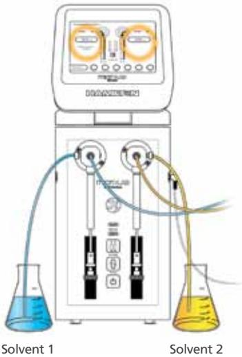
**Step 2.** Trigger the hand probe to fill the left and right syringes with Solvents 1 and 2.
