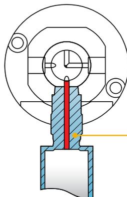
Traditional TLL syringes trap approximately 50  $\mu\text{L}$  of air, making small syringes nearly impossible to prime.
