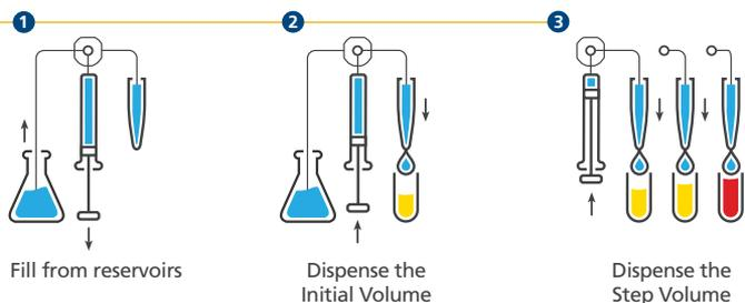
A large Initial Volume is dispensed to get close to the endpoint. Then a smaller Step Volume is dispensed until the endpoint is reached.
