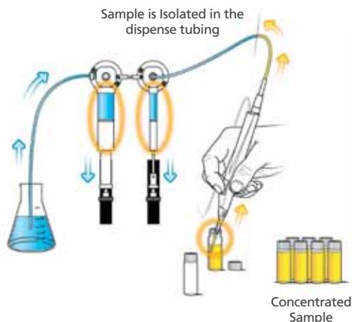
**Step 3.** Trigger the hand probe to dispense the Sample and then Diluent into a vial.
