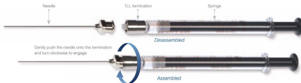
Figure 1. Assembly of Metal Hub Needle onto TLL Syringe
