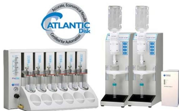
The Horizon Technology SPE-DEX® 4790 Automated Extraction System, Envision® Platform Controller, and DryVap® Automated Drying and Concentrating System.
