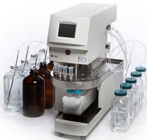
The Horizon Technology SmartPrep<sup>®</sup> Automated Cartridge Extractor
