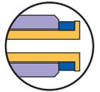
For those systems requiring or preferring flanged connections, use these fiberglass-reinforced fittings with our Easy-Flange flanging tool and polypropylene washers to make a clean connection. The flange on the tubing ensures that the washer never comes in contact with the mobile phase.
