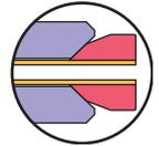
A unique mixing results from the turbulence created by the introduction angle of the solvents. The mixing is much more thorough than with a conventional tee.
