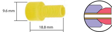
Polyacetal flangeless nuts in combination with the inverted ferrule do not require a flanging tool. A hand-tightening procedure makes leak-free seals. With this fitting system, the inert ETFE ferrule is the only part besides the tubing which comes into contact with the fluid stream – the nut is never in contact. Six colors are available.
