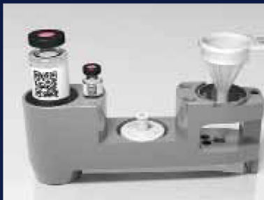
2. Load flow cell into puck
