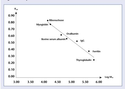
$K_{av}$  (partition coefficient) is plotted against the logarithm of molecular weight for selected proteins. The selectivity curve is straight over the range  $K_{av}$ =0.2 to  $K_{av}$ =0.8. Here, the dimer of thyroglobulin elutes in the void volume  $V_0$  ( $K_{av}$ =0) and the other proteins nicely follow the theoretical  $K_{av}$  curve.
