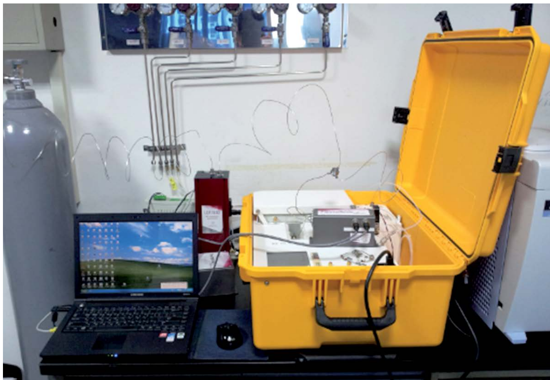
Figure 5: PlasmaDetek installed in a portable unit
