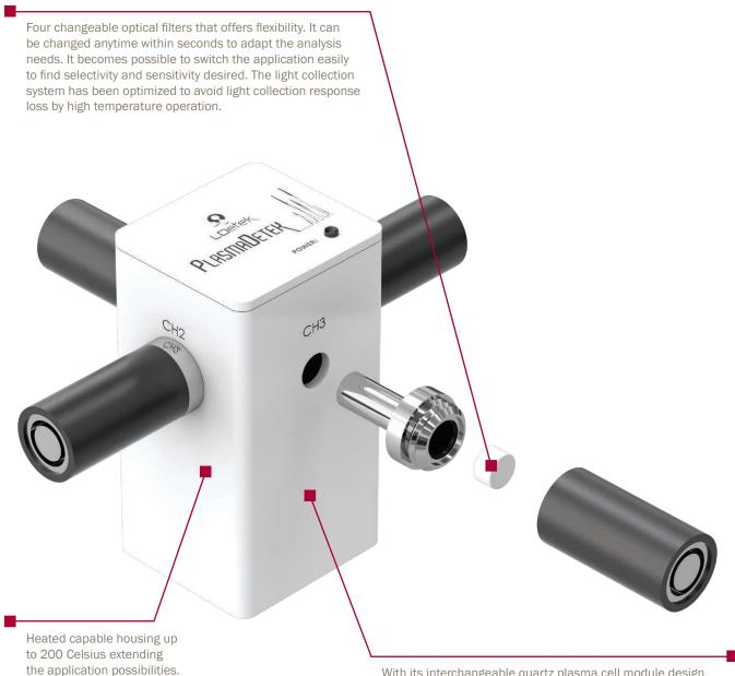
With its interchangeable quartz plasma cell module design, it becomes possible to do the maintenance on the detector. The application can be modified easily as well. The detector module design makes it easy to replace or change any component without damaging or creating leaks. The design offers an integrated leak detector to auto diagnostic the carrier gas and make up leak rate.
