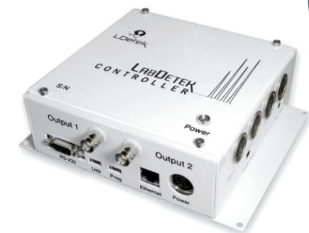
The LabDetek controller is used with the platform. This device offers multiple I/Os that can be used for different tasks like signal acquisitions, valves actuation, ovens and flows control. The controller communicates with the LabDetek interface module using Clarity from DataApex. The controller also offers serial and LAN communication protocols.
