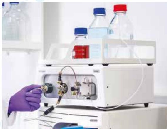
A compact liquid sampling interface, our optional MiDas™ module allows automated sampling, dilution and injection for direct mass spectrometer analysis at the point of reaction or during processing.
