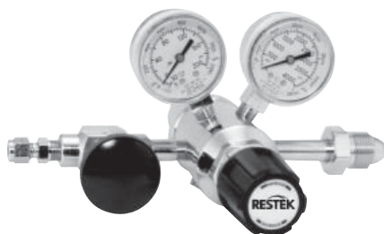
Inlet gauge: 0 to 4,000 psig (0–27,579 kPa) Outlet assembly: diaphragm valve, 1/4" tube fitting
