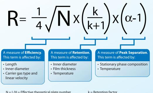
N = L/H = Effective theoretical plate numberL = Column length H = HETP = Height equivalent to a theoretical plate
