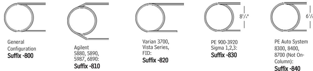
**Note:** Initial 2" of column will be empty, to accommodate a needle. For a completely filled column add suffix -901.
