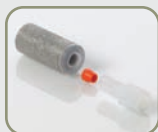
11-1422 Solvent Filter 10µm SS with 1/4-28 Nut/Ferrule for 3mm OD Tubing
