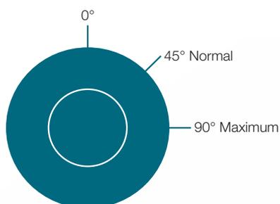
**Step 1:** Connect the column by carefully tightening the nanoViper connection until the point of first resistance (also known as 0° mark).
