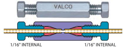
Standard bore – ends of tubing seat squarely at bottoms of fitting details (ZU1)
