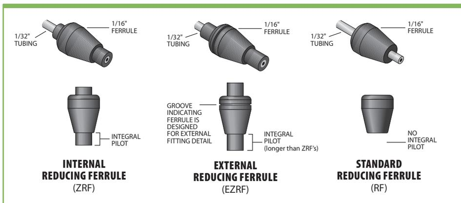
dead volume fitting. A single groove indicates that the ferrule is for use in an external detail.
