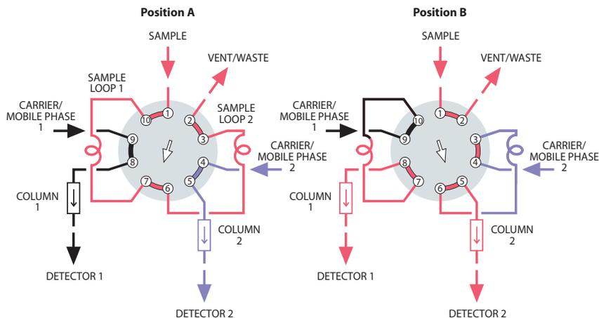
**SIMULTANEOUS INJECTION OF THE SAME SAMPLE ONTO SEPARATE COLUMNS**
