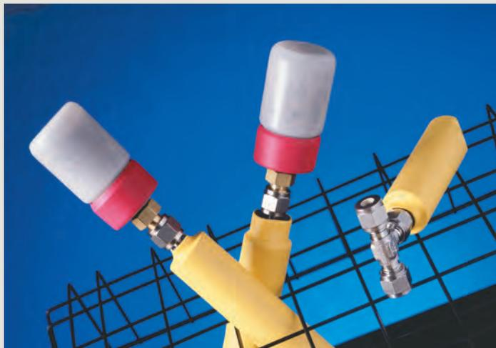
Over 100 different substances are available, including Arsine, Phosphine, and gas phase devices such as CO, NO, and Methane. Available permeation rates range from less than 100 ng/min to 50,000 ng/min. Each G-Cal device is individually calibrated and verified to generate a given mass output per unit time (ng/min) at a set point temperature. A graph which shows an estimated permeation rate vs. temperature from 0 to 50°C is included with each device.
