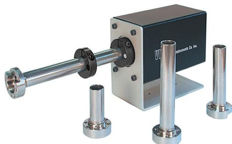
Valves which will be installed in ovens or heated zones require a standoff assembly, which locates the actuator out of the heated zone and supports both the valve and the handle or actuator. The 5/8" outside diameter standoff tube extends through the oven wall and is secured by means of a clamp ring supplied with the assembly.
