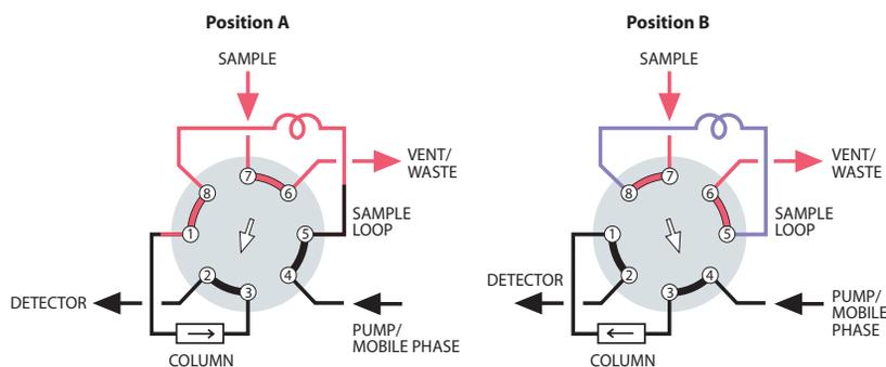
**LOOP SAMPLING WITH BACKFLUSH TO DETECTOR**
