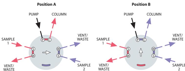
DUAL MICROVOLUME SAMPLE INJECTION
