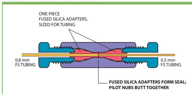
For connection of fused silica tubing of the same or differing sizes, the **through-bore union** shown in **FIGURE 9** is recommended. This fitting permits the use of our one-piece fused silica adapters to effect a true zero dead volume connection. The ferrule features an integrated pilot which adapts to the ID of the unions, resulting in an inert, zero volume connection.
