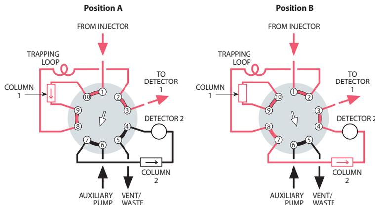
HEART CUT TRAPPED IN A LOOP AND INJECTED ONTO A SECOND COLUMN
