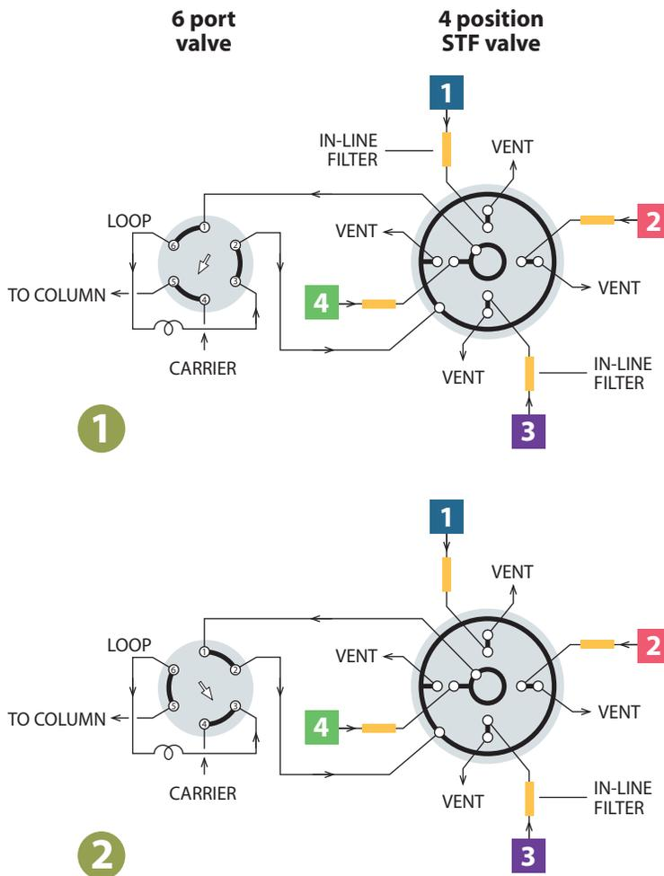
**SAMPLE TRAPPING WITH CONTINUOUS FLOW TO INDIVIDUAL OUTLETS**
