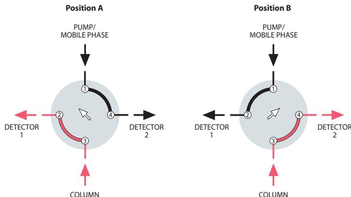
**DETECTOR SELECTION FROM TWO COLUMNS OR ONE COLUMN AND AUXILIARY CARRIER**
