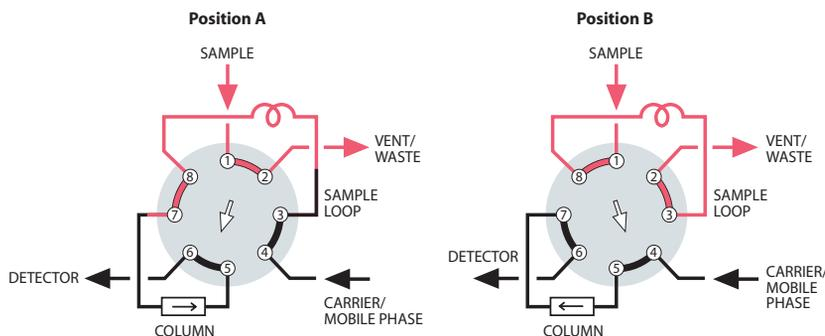
**LOOP SAMPLING WITH BACKFLUSH TO DETECTOR**
