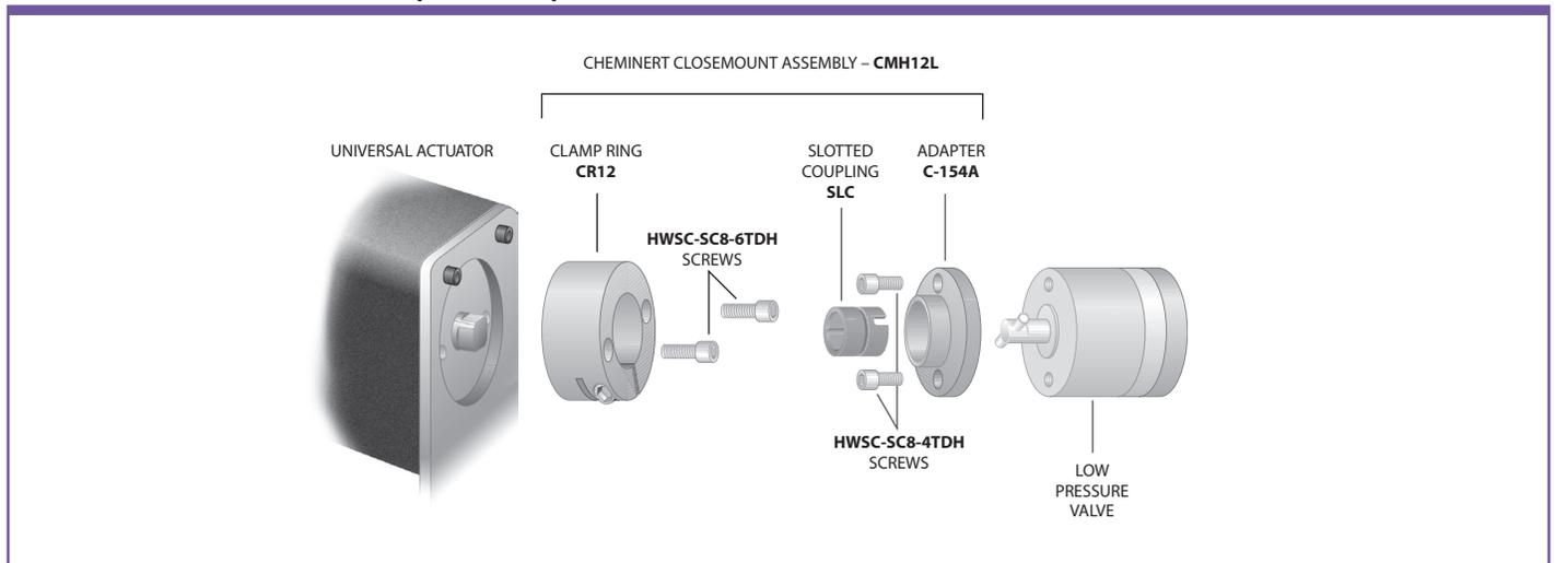
**CLOSEMOUNT – VALCO VALVE (1 or 2 mounting holes) – AIR ACTUATOR**
