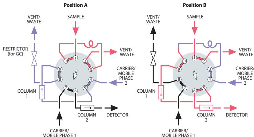
**LOOP SAMPLING WITH BACKFLUSH OF PRE-COLUMN TO VENT**
