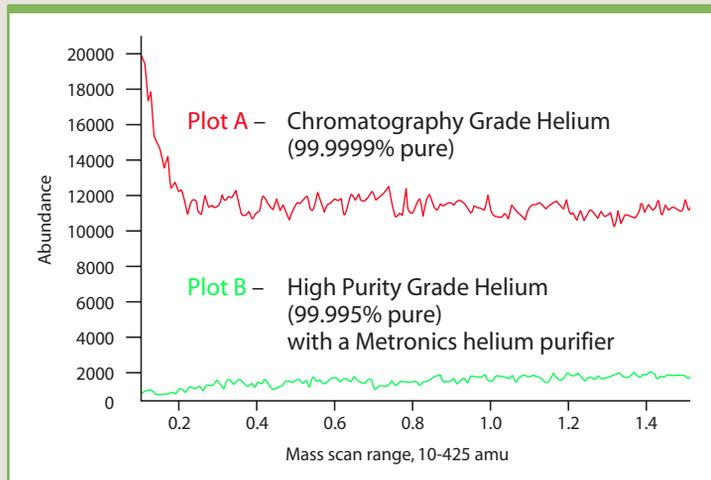
produce gases that are at least a factor of ten higher than a 99.9999% “chromatography grade” cylinder of gas when the purifier is supplied by a 99.995% cylinder. The cost difference between the two grades of gas will pay for the cost of the gas purifier several times over during its operating life.
