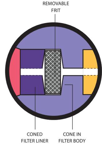
**FILTER WITH FRIT REMOVED BEING USED AS A REDUCING UNION**
