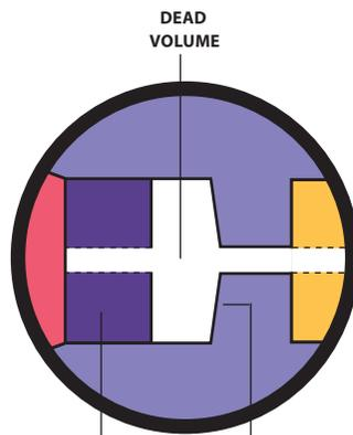
TUBE MADE UP IN A STANDARD UNION      CONE IN FILTER BODY
