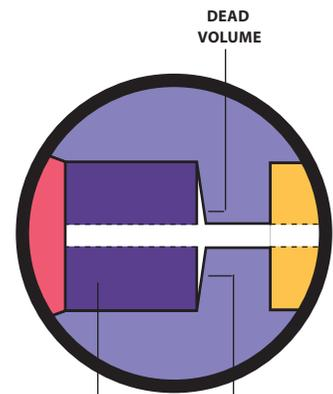
TUBE MADE UP IN A FILTER      CONE IN FILTER BODY
