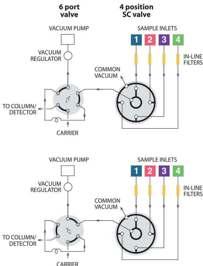
STREAM SELECTION WITH CONTINUOUS FLOW TO A COMMON OUTLET
