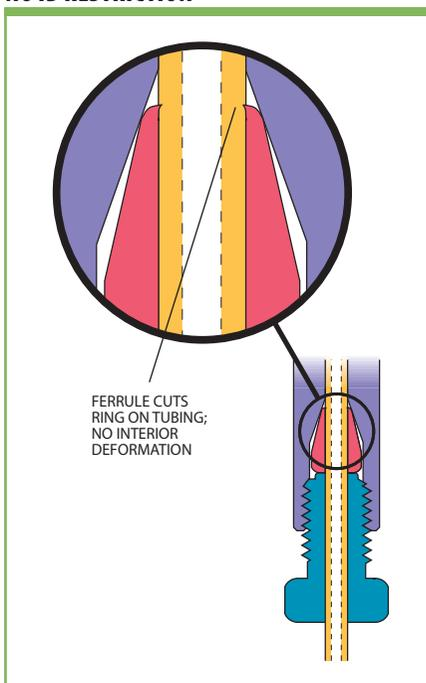
designed for a slightly longer tube extension (as in **FIGURE 4B**), dead volume will be introduced. In the opposite case, with the pilot shorter than the pilot depth (**FIGURE 4C**), the tube will bottom out before the ferrule has sealed. However, our tests prove that except in the most extreme cases, a Valco ferrule will "creep" on the tubing until it reaches the bottom of the ferrule taper, making a proper seal.
