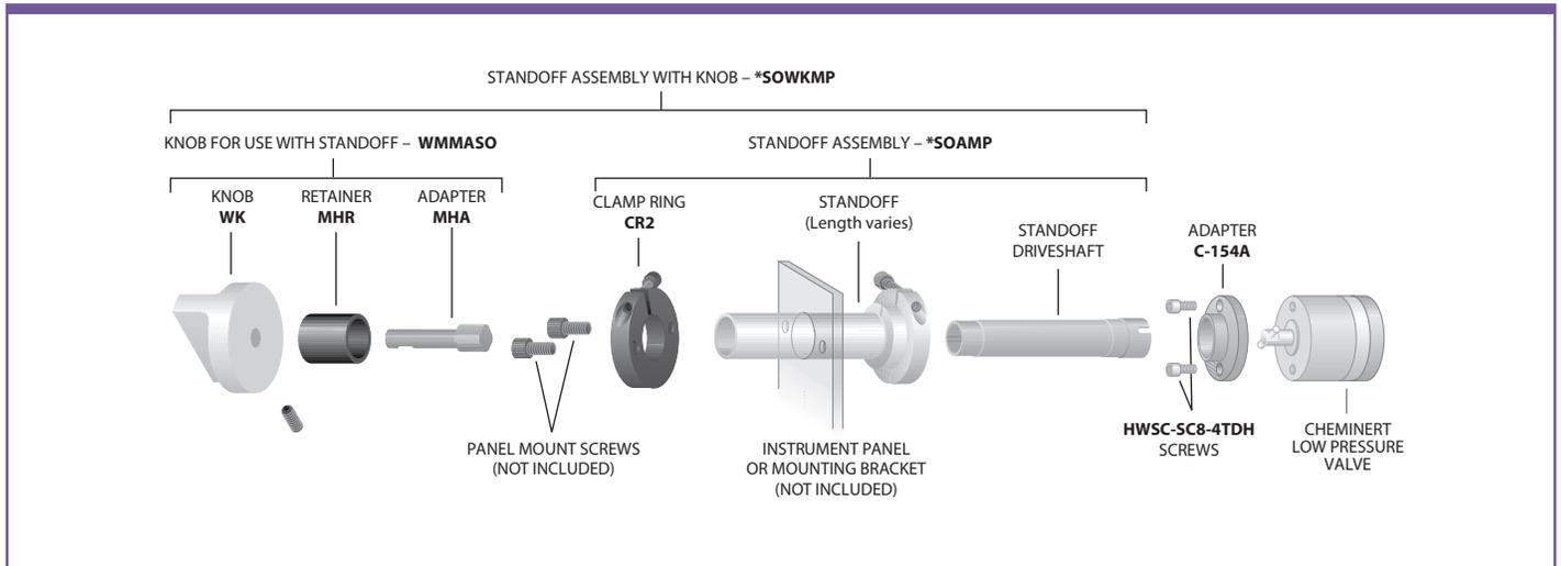
**KEYED S TANDOFF– CHEMINERT SELECTOR – UNIVERSAL OR MICROELECTRIC ACTUATOR**
