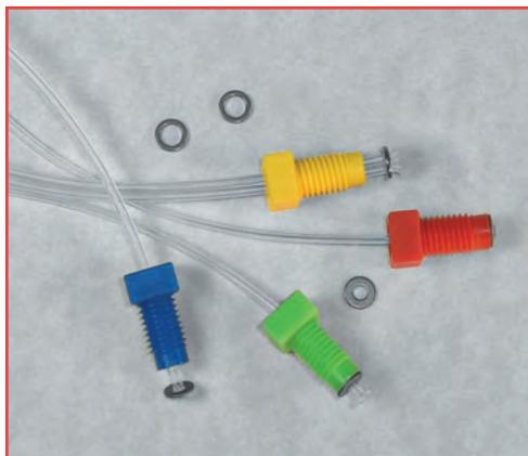
The basic component of the Cheminert system is the polypropylene nut, retained on PTFE or FEP tubing by a flange formed with a Cheminert flanging tool (page 54). This is an excellent method for connecting fluorocarbon tubing, as there is no reduction of the inside diameter and no binding or twisting of the tubing when the fitting is tightened. A mating of the parts is achieved with zero dead volume, making this an ideal fitting for biological systems.
