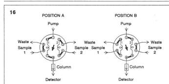
A. Fill sample loop 2 with sample 2. Inject sample loop 1 into column.
