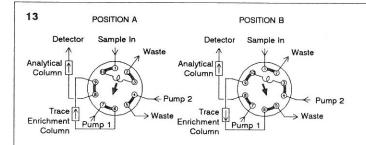
A. Fill sample loop with waste water.
